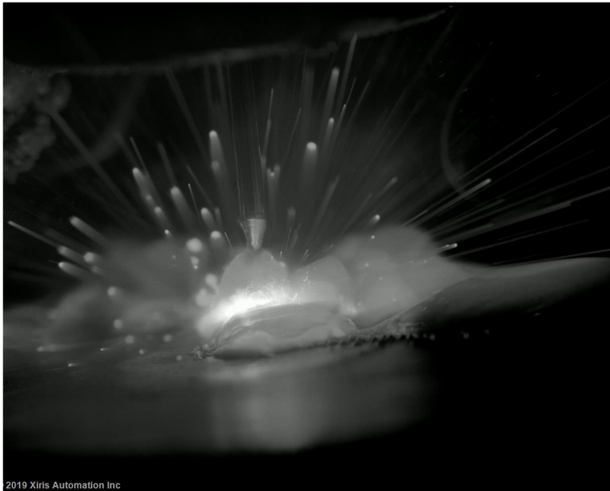
Short Circuit GMAW at point of expulsion
